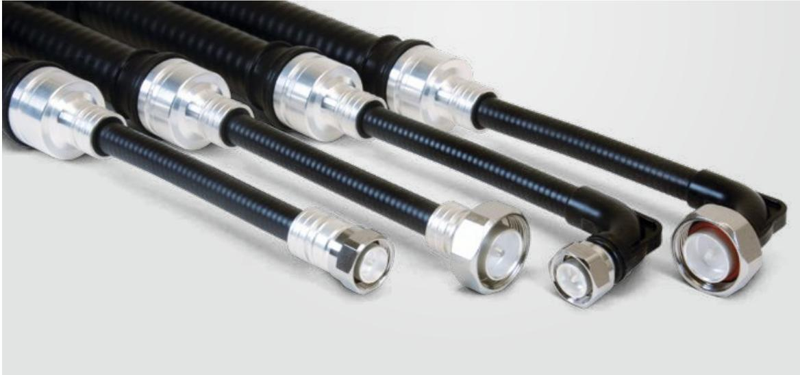
The SpinnerFlex® Hybrid jumpers are based on SF 1/2" and LF 7/8" cable and available with 7-16, 4.3-10, 4.1-9.5, N or 2.2-5 connectors. Total length is between 6 and 20 meters, the SF 1/2" jumper part is one meter on each side. Other versions can be made available on request.
