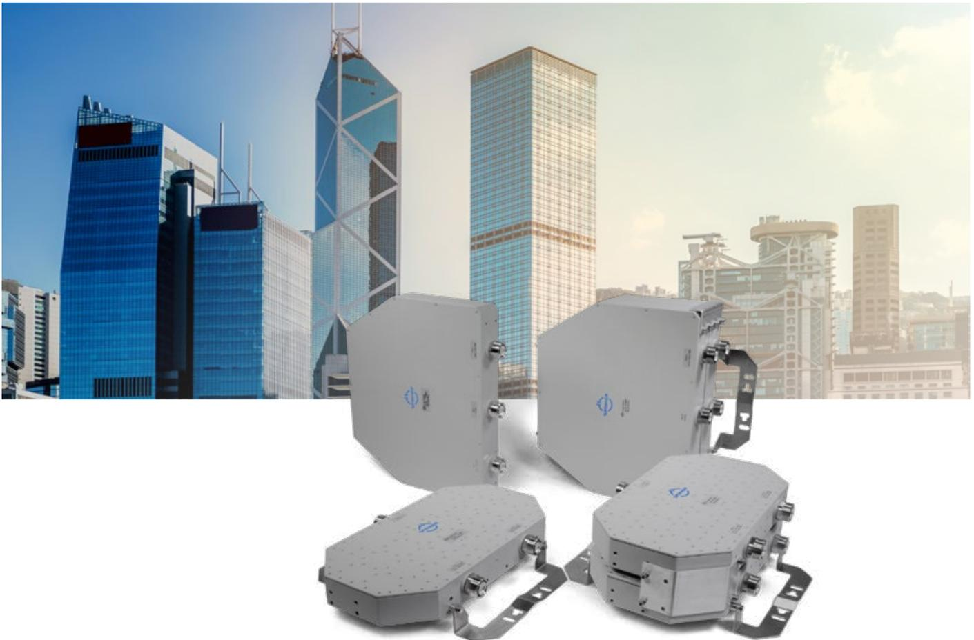
Sameband combiners enable antenna and feeder sharing for two or more base stations in the same frequency band. For this purpose, the transmitted and received signals of base stations are separated and the corresponding signals are combined via band-pass filter and star points. SPINNER sameband combiners stand out for low insertion loss, high isolation between frequency blocks and extremely low intermodulation.
