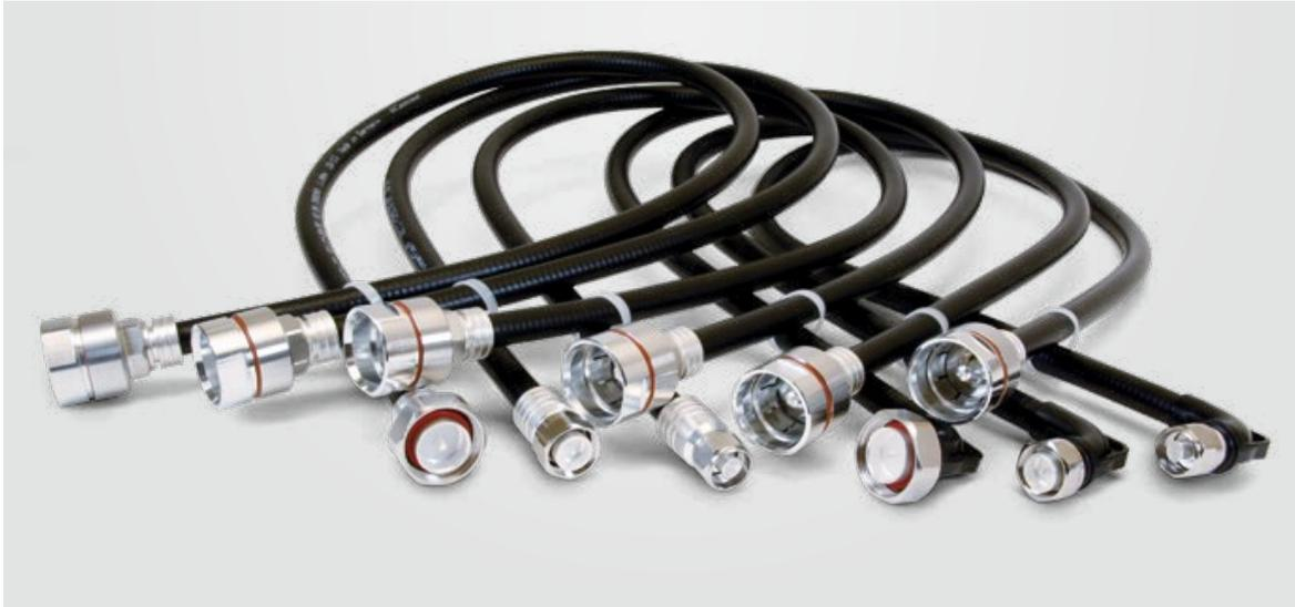
SpinnerFlex® MultiFit jumpers are based on SF 1/2" jumper cable. On one end fits a LF 7/8" feeder connector/cable clamp, the other end can be fitted with 7-16, 4.3-10, 4.1-9.5, N or 2.2-5 connectors.
