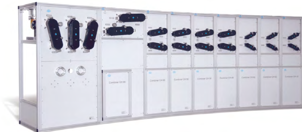
BN 575306 Turkmenistan UHF combiner for 8 x 4 kW DVB with integrated mask filters, combiner bypass and antenna patch panel with bent front for installation in circular transmitter hall
