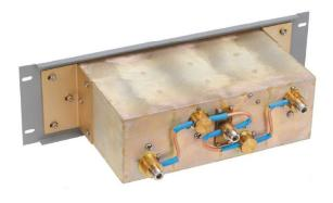
EN Series Antenna Duplexers consist of a group of cavity resonators connected and tuned together to allow both a transmitter and a receiver to share a common antenna allowing bi-directional (duplex) communication over a single channel. These units feature compact, high Q cavities, requiring less rack space than standard 4-inch cavities. The cavities are arranged in an order which provides enough isolation to keep the transmitter from interfering with the receiver.
