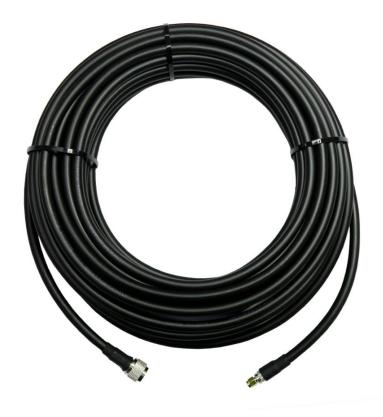
The 1012096 is a prepared Co-axial lead of 20m of LL400 Cable with one N Plug termination and one SMA Plug termination. Both connectors have glue type heatshrink protecting cable entry from the weather.
