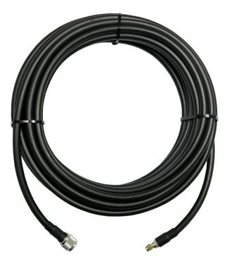
The 1012095 is a prepared Co-axial lead of 12 M (40 FT) of LL400 Cable with one N Plug termination and one SMA Plug termination. Both connectors have glue type heatshrink protecting cable entry from the weather.
