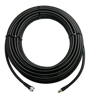
The 10120949 is a prepared Coaxial Lead of 10 M (60 FT) of LL400 Cable with one N Plug and one SMA Plug termination. Both connectors are fitted with a Heatshrink sleeve to ensure protection.
