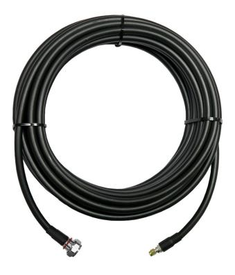
The 10120948 is a prepared Coaxial lead of 10 M (33 FT) of LL400 Cable with of LL400 Cable with one 4.13-10 Plug termination and one SMA Plug termination. Both connectors have glue type heatshrink protecting cable entry from the weather.
