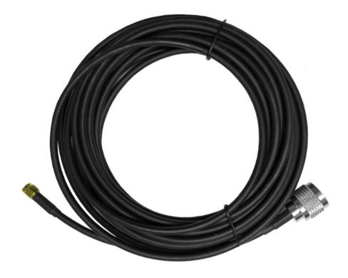
The 101208 is a prepared Coaxial Lead of 2m in length. It uses Benelec 056031 LL195 low loss coaxial cable with 04206 N-types male crimp plug at one end and a 040013 SMA male plug at the other. Both connectors have Heatshrink protecting cable entry.
