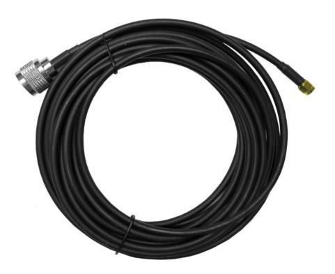
The 101205 is a prepared Coaxial lead of 6 M (18 FT) in length. It uses Benelec 056031 LL195 low loss coaxial cable with a 04206 N-type male crimp plug at one end with a 040013 SMA male plug at the other. Both connectors have glue type heat shrink protecting cable entry from the weather.
