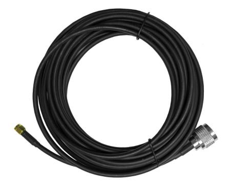
The 101205 is a prepared Co-axial lead of 6 M (18 FT) in length. It uses Benelec <u>056031</u> LL195 low loss coaxial cable with a **04206** N-type male crimp plug at one end with a **040013** SMA male plug at the other. Both connectors have glue type heatshrink protecting cable entry from the weather.
