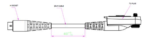
07890T1 is a H socket to T1 termination. Supported radio model with this socket is mentioned below.
