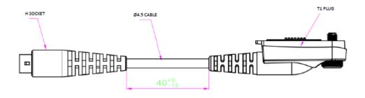
07890T1 is a H socket to T1 termination. Supported radio model with this socket is mentioned below.
