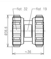
The 048610S is a 7-16 DIN Plug to 7-16 DIN Plug Adaptor. This connector has a silver-plated inner and CuSnZn plated outer conductor. This connector is IP68 rated.
