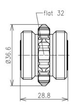
The 0485142S is a 7-16 DIN Socket to 7-16 DIN Socket Adaptor. This connector has a silver-plated inner and outer conductor. PTFE insulator and silicon rubber sealing are provided for protection.
