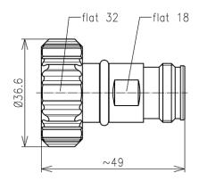
The 048509S is a 4.3-10 DIN Socket to 7-16 DIN Plug Adaptor. This connector has a silver-plated inner and CuSnZn - plated outer conductor. This connecter is IP 68 rated.
