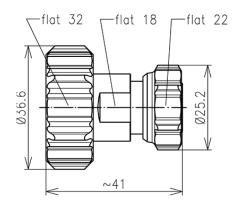
The 048508S is a 4.3-10 DIN Plug to 7-16 DIN Plug Adaptor. This connector has a silver-plated inner and CuSnZn - plated outer conductor. This connector is IP68 rated.
