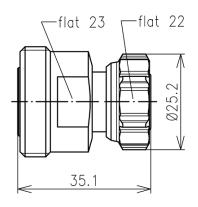
The 048507S is a 4.3-10 DIN Socket to N Socket Adaptor. This connector has a silver-plated inner and CuSnZn plated outer conductor. This connector is also IP68 rated.
