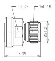
The 048505S is a 7-16 DIN Socket to N Plug Adaptor. This connector has a silver-plated inner and outer conductor. PTFE insulator and silicon rubber sealing are provided for protection.
