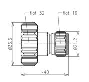
The 048504S is a 7-16 DIN Plug to N Plug Adaptor. This connector has a silver-plated inner and outer conductor. PTFE insulator and silicon rubber sealing are provided for protection.
