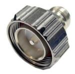
The 048503S connector is a 7-16 DIN Plug to N Socket Adaptor. This connector has a silver-plated inner and outer conductor. PTFE insulator and silicon rubber sealing are provided for protection.
