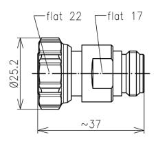
The 0483122S is a 4.3-10 DIN Plug to N Socket Adaptor. This connector has a silver-plated inner and CuSnZn plated outer conductor. PTFE insulator provides protection.
