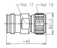
The 0483120S is a 4.3-10 DIN Socket to N Plug Adaptor. This connector has a silver-plated inner and CuSnZn plated outer conductor. PTFE insulator and silicon rubber sealing are provided for protection.
