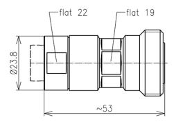
The 048105MLS is a 7-16 DIN Socket for 1/2" Feeder. This connector has a silver-plated inner and CuSnZn plated outer conductor. PTFE insulator and silicon rubber sealing are provided for protection.
