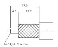
04809 is a 7-16 DIN Plug and includes a spring finger centre and crimp outer sleeve. This connector has a silver-plated centre pin, nickel-plated body, coupling cap, and ferrule. PTFE insulator and silicon rubber gasket are provided for protection.
