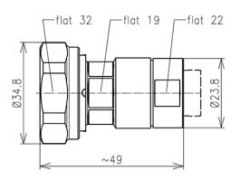
The 048005MLS is a 7-16 DIN Plug for 1/2" Feeder. This connector has a silver-plated inner and CuSnZn plated outer conductor. PTFE insulator and silicon rubber sealing are provided for protection.
