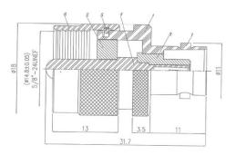
The 04372 is a BNC Socket to UHF Plug Adaptor. This connector has a gold-plated centre pin and nickel-plated body. Two Teflon material insulators are provided for protection.
