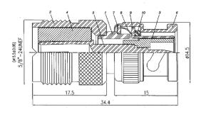
The 04371 is a BNC Plug to UHF Socket Adaptor. This connector has a gold-plated centre pin, nickel-plated body, washer, and retaining ring. Two Teflon material insulators and one rubber gasket are provided for protection.
