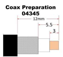
The 04345 BNC socket is a crimp inner – crimp outer solder style, although it can be used as solder inner, crimp outer. It is a quality Nickel plated product with gold finish on the centre pin contact & also the soldering surface (inside of centre pin). Unlike silver plated connectors it has high resistance to tarnishing.
