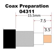
The 04311 BNC plug is a crimp inner – crimp outer solder style, although it can be used as solder inner, crimp outer. It is a quality Nickel plated product with gold finish on the centre pin contact & also the soldering surface (inside of centre pin). Unlike silver plated connectors it has high resistance to tarnishing.
