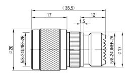
04282 is an N Plug to UHF Socket. This connector has a silver-plated conductor and nickel-plated body with an ABS insulator.
