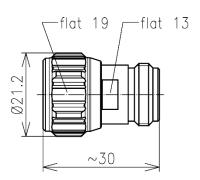
The 04251S is an N Plug Adapter to N Socket Port Saver. This connector has a silver-plated inner and outer conductor. PTFE insulator and silicon rubber sealing are provided for protection.
