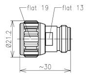
The 04251S is an N Plug Adapter to N Socket Port Saver. This connector has a silver-plated inner and outer conductor. PTFE insulator and silicon rubber sealing are provided for protection.
