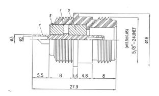
The 04230 is an N socket panel, no flange type connector. It has solder pot contact. The centre pin is gold-plated, and the body is nickel-plated.
