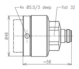
The 042108MLS is a N Socket for 1 1/4" Feeder Cable. This connector has a silver-plated inner and CuSnZn - plated outer conductor. PTFE insulator and silicon rubber sealing are provided for protection.
