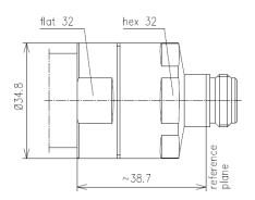
The 042107MLS is an N socket-type connector. It has a gold-plated inner conductor and a nickel-plated outer conductor. This connector also has a silicone rubber for sealing and protection.
