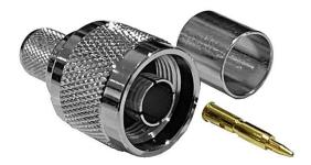
The 04208 is an N plug connector with a gold-finished centre pin and nickel-plated body. Soldering is required for connecting the gold-plated centre pin. It also has a nickel-plated washer, nut, ferrule, and gasket.
