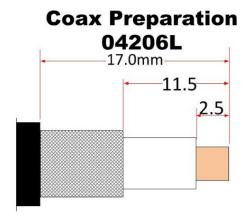
The **04206L Right Angle N-type** *plug* is a commercial quality solder centre, crimp outer style. It is a quality nickel plated product with a gold finish on the centre pin contact & also the soldering surface (inside of centre pin). Unlike silver plated connectors it has high resistance to tarnishing. The shield is crimped.
