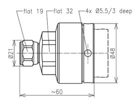
The 042008MLS is a N Plug for 1 1/4" Feeder Cable. This connector has a silver-plated inner and CuSnZn - plated outer conductor. PTFE insulator and silicon rubber sealing are provided for protection.
