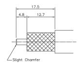
The 04169 is a spring finger centre and crimp outer TNC connector. It has a gold-finished centre pin, nickel-plated body, ferrule, and coupling cap.
