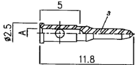
04161 is a TNC connector with a gold-finished centre pin and nickel-plated body. Soldering of the centre pin is required.
