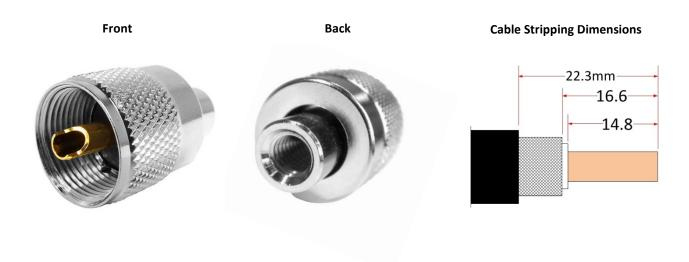
The 04104 UHF PL-259 plug is a combination screw-on & solder style. It is a quality Nickel plated product with Gold finish on the centre pin contact & also the soldering surface (inside of centre pin). Unlike silver plated connectors it has high resistance to tarnishing.
