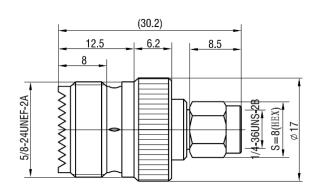
The 0400410 is a SMA Plug to UHF Socket Adaptor. This connector has a gold-plated centre pin and nickel-plated body. Teflon insulator is provided for protection.
