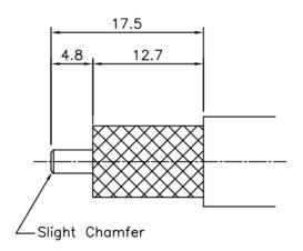
The 040014 SMA-type plug is a commercial quality spring finger coaxial connector. It is a quality Nickel plated product with Gold finish on the centre pin contact & there is no soldering or crimping required for the centre conductor, as the spring finger captivates the cable as it is pushed into the connector. Unlike silver plated connectors it has high resistance to tarnishing.
