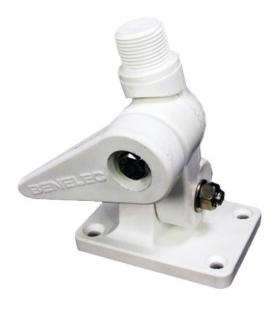
An adjustable antenna mount that articulates for horizontal, vertical or inclined mounting surfaces. It is entirely constructed of glass filled nylon, lightweight & suited to shipboard and fixed station applications. The male mounting thread is the Marine standard 1" 14tpi.
