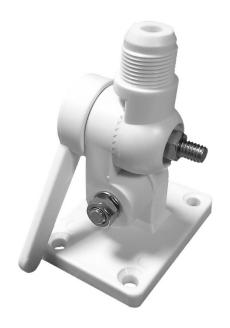
An adjustable antenna mount that articulates for horizontal, vertical or inclined mounting surfaces. It is entirely constructed of nylon, lightweight & suited to shipboard and fixed station applications. The male mounting thread is the Marine standard 1" 14tpi.
