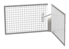
The model 02688Q is a heavy duty 90 degree corner reflector antenna, ideally suited to applications where a high front to back ratio and forward gain are required. This antenna is ideal for reducing unwanted interference from other communication sites whilst maintaining a strong forward signal. The Stainless Steel construction is ideally suited to harsh environment locations. This antenna comes in a disassembled state and can be assembled on site.
