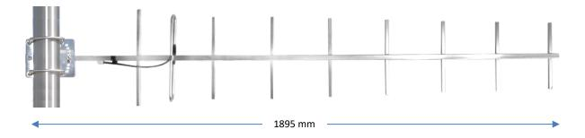
The 02683Q Yagi antenna is a 11dBd Gain 9 element all Stainless-Steel directional Yagi antenna for use in the 370 – 400 MHz radio band. Its gain affords excellent radio link coverage. The robust construction ensures excellent longevity and performance. The Electropolished all Stainless-Steel construction is ideally suited for weather and corrosion resistance. All mechanical connections are welded for minimum inter-modulation levels. All electrical connections are directly soldered.
