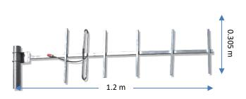
The 02682W antenna is a 9.0dBd Gain, Yagi antenna for use in the Commercial Radio Band. Its high gain affords exceptional radio link coverage. The 02682W antenna offers a stable radiation pattern across the whole band 450 - 480 MHz Its robust construction ensures excellent longevity and performance.
