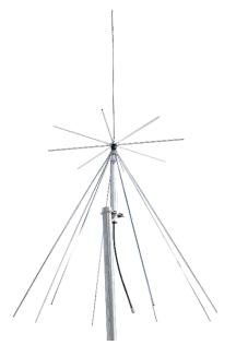
The 02674 is a receive Antenna, for use across the 65 - 1300 MHz Radio Band. It can also be used as a transmit antenna in selected bands, as outlined in the table below. It is manufactured with removable Stainless Steel radials, making it suitable to applications where rapid deployment is required. It can also be used satisfactorily for permanent installation. Heavy Duty stainless steel construction will lead to long term reliable service by this antenna.
