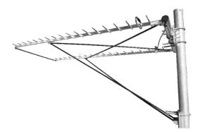
The 024872 yagi antenna is a 18.8dBi Gain 18element all Stainless Steel two stack directional yagi antenna array for use in the 804-854MHz radio band. Its gain affords excellent radio link coverage.
