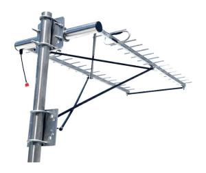
The 024842 yagi antenna is a 15dBd Gain 15element all Stainless Steel two stack directional yagi antenna array for use in the 800-896MHz radio band. Its gain affords excellent radio link/4G coverage\*.
