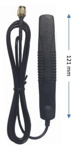
The 024571G is an economically priced, compact, medium gain 5G antenna suited for use in the bands 690 - 960 & 1710 - 2700 & 3500 - 3700 MHz. It comes standard with flexible 1.5 meters of low loss cable terminating in an SMA male connector & is suited for mounting onto a wall bracket.
