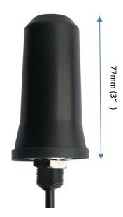
The 024563 is an economically priced, compact, unity gain 5G antenna suited for use in the frequency bands 695-960, 1710-2700, 3500-3800 MHz. It comes standard with 2 m (6 ft) of low loss cable terminating in an SMA plug connector and is suited for mounting onto telemetry boxes. Comes with "L" Bracket.
